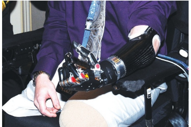
Air Force Tech Sgt. Joe Deslauriers is learning the intricacies of his new arm. The DEKA arm has 10 degrees of movement. Photo courtesy of Rob McIlvaine.
